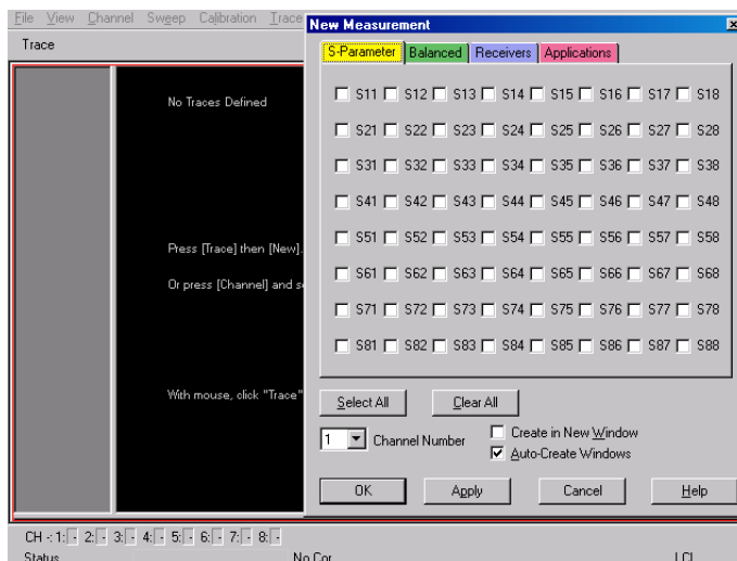
Figure 17 12-Port New Trace Measure (S11 - S88)
